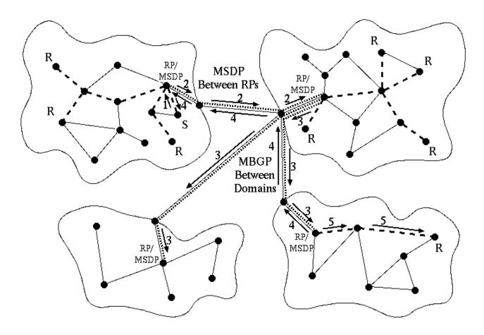
Figure 5: MSDP operation including flow of Source Active (SA) messages.
