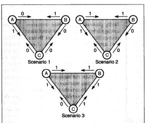
Figure 10. Scenarios leading to failure of Byzantine agreement.
