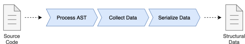
Figure 5.1: Steps of the collector when retrieving structural information from source code.
