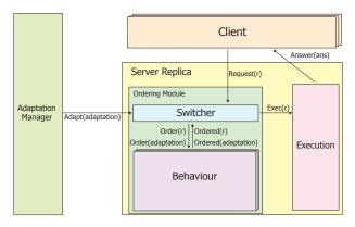
Figure 1: System architecture
