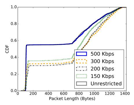
Figure 5.9: Packet length CDF of a reference stream varying the connection bandwidth.
