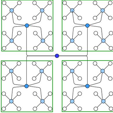
Fig. 4: Cloudlet placement (white) and broker network (blue)
