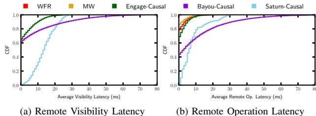
Fig. 7: CDF of the Remove Visibility Latency and Remote Operation Latency.
