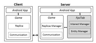
Figure 5: Overall system architecture.
