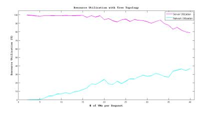
Fig. 5. Resource utilization using a Tree topology.
