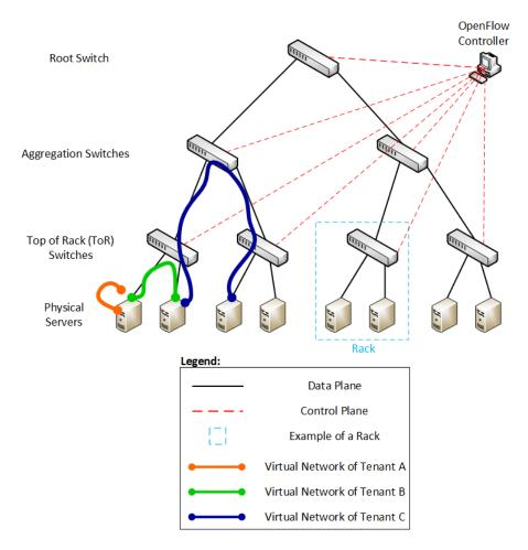
Fig. 1. High level architecture of the solution with a tree topology.
