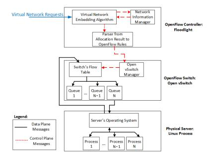
Fig. 2. Software architecture of the components present in the solution.
