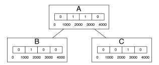
FIGURE 2.4: Example bitmap indexes, as used in [27], to represent CPU Speed (in MHz) in nodes B and C, along with aggregated information (bitwise OR) in parent node A.
