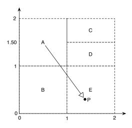
FIGURE 2.3: Example CAN coordinate space of [0,2]x[0,2]. Nodes B, C, and D are node A's neighbors. Query for key that maps to (1.3, 0.3), starting from node A, is routed first through B and then finally to E, which is responsible for that zone.
