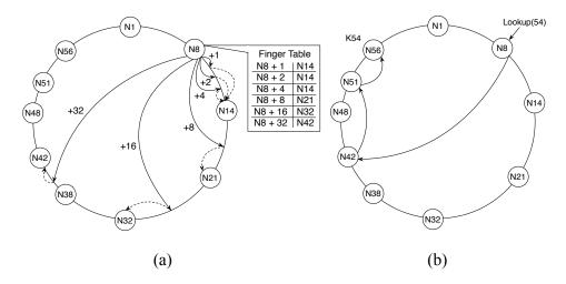
FIGURE 2.2: (a) Example finger table for node 8. (b) Routing of query for key 54 using the finger table to speedup lookup.
