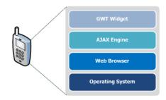
Figure 5: Client Component's Architecture
