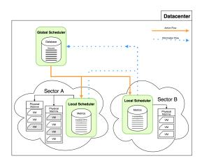
Figure 2: High-level architecture
