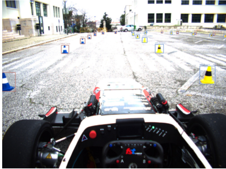
Figure 2.3: YOLOv5 applied to a frame on Autonomous Driving.
