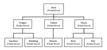
Figure 3: The conceptual representation of a DirectoryTree stored by the Metadata Manager for each Briefcase. In this image the Root folder represents a Briefcase. The Root's FolderStruct has a list that contains three other FolderStructs, each for a different of its sub-folders (Images, Videos and Music). Similarly, each of these sub-folders also contains a list that stores FolderStructs representing its subfolders.
