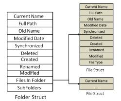
Figure 2: The image represents the FolderStruct and the FileStructs stored within. The FolderStruct is a structure that contains important information concerning a certain folder. A FileStruct on the other hand contains information concerning a file. This information is used by the Resolver during the synchronization process.
