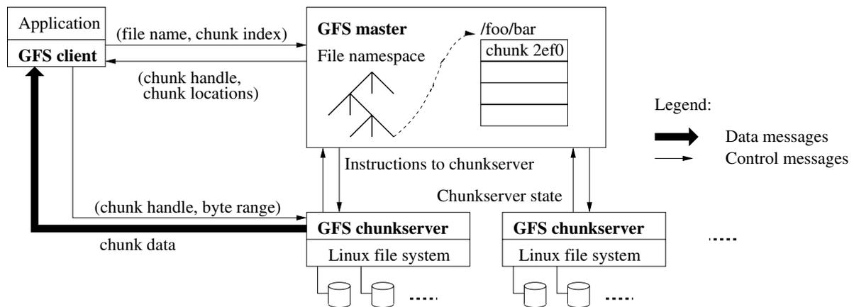
Figura 2.1: The Architecture of GFS (Ghemawat et al. 2003)
