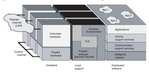
Figure 3 Architecture and interconnection of CRUTIAL nodes (e.g. CIS)
