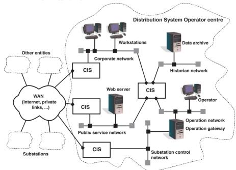
Figure 2 Example mapping of part of an infrastructure to the WAN-of-LANs architecture
