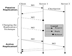
Figure 7. Interceptor actions during reconfiguration.
