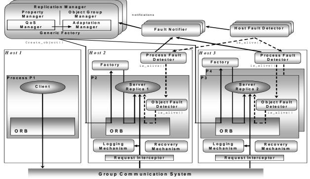
Figure 1. Adaptive Fault-Tolerant Architecture.
