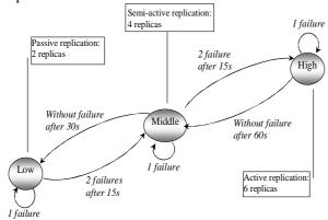
Figure 2. State machine of the QoS Manager.
