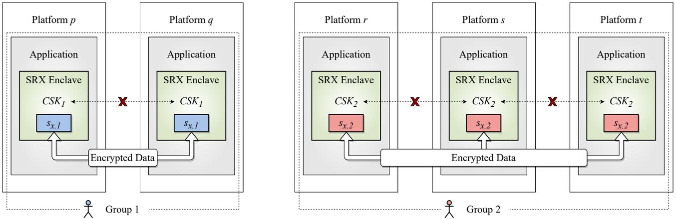
FIGURE 1. High-level view of SRX depicting two distinct groups of platforms. Platforms in Group 1 share SRX sealed data with one another, without exposing their Common Sealing Key ( $CSK_1$ ) outside the respective enclaves, but not with platforms in Group 2 which have their own Common Sealing Key ( $CSK_2$ ).
