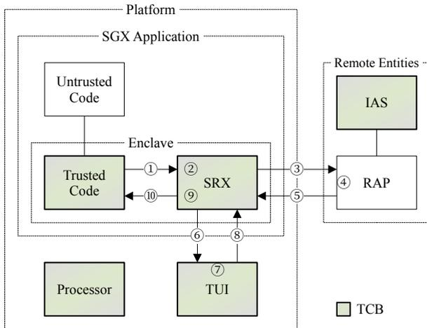
FIGURE 2. Typical architecture of a system using the SRX trusted library. The circled step numbers are used in the protocols' description (§ III).
