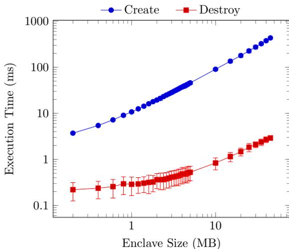
FIGURE 9. Execution time for creating and destroying an enclave.
