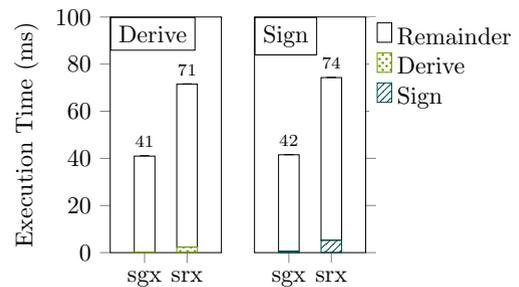
FIGURE 5. Total execution time of operations *derive* and *sign* of the bitcoin wallet. The remainder block includes the enclave life cycle.
