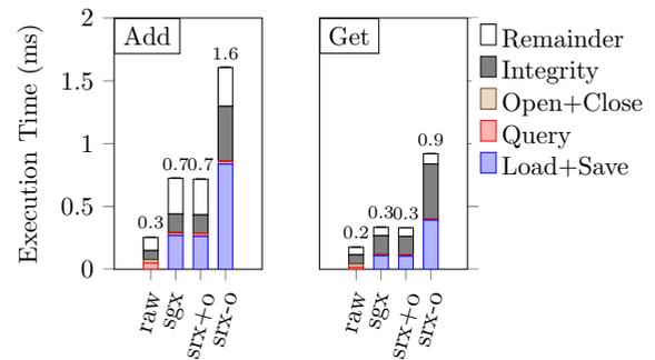
FIGURE 8. Execution time of functions *add* and *get* of the password manager.
