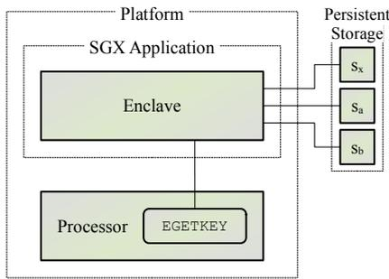
FIGURE 3. Storage of sealed data  $s_a$  of the application enclave and  $s_x$  of SRX.
