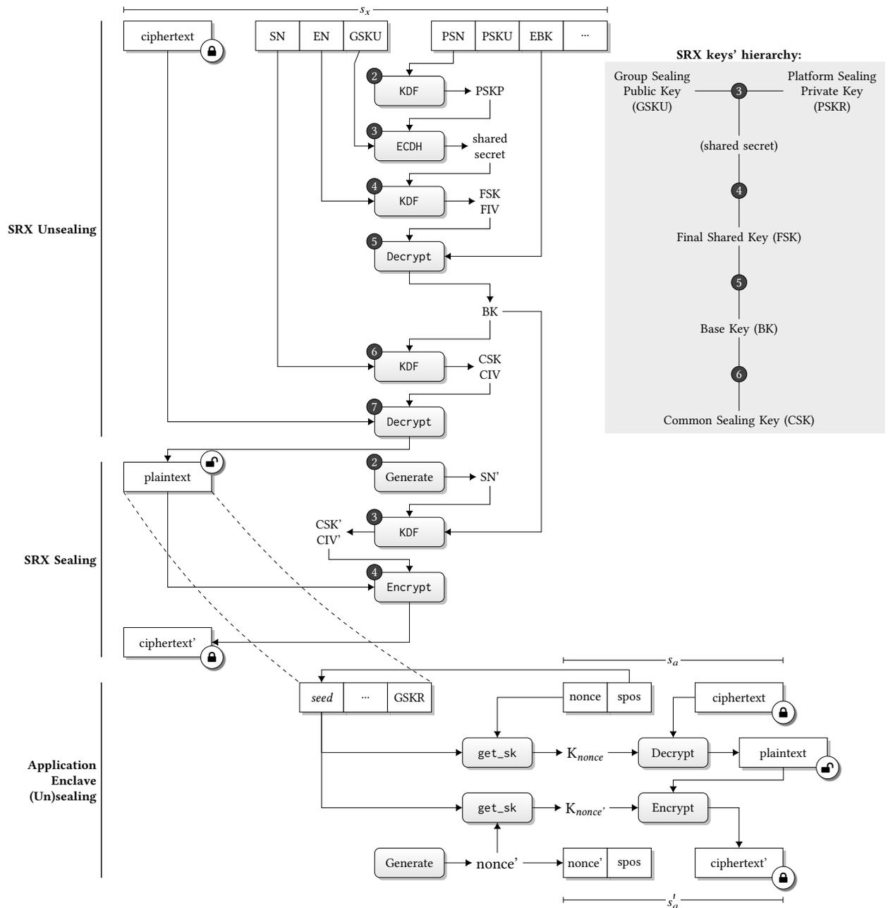
**FIGURE 10.** Derivation of keying material for unsealing, and sealing,  $s_x$  and  $s_a$ . Steps 2–7 in *SRX Unsealing* and 2–4 in *SRX Sealing* match line numbers in Algorithm 1 and Algorithm 2, respectively. The hierarchy between the SRX keys is shown on the top-right and the numbers match the steps in the function boxes.
