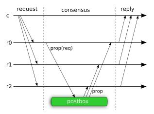
Figure 6. SMIT algorithm steps sequence
