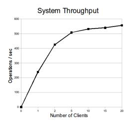
Figure 7. Throughput under different loads
