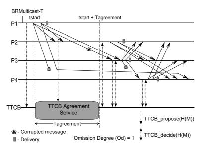
Figura 3: Example execution of the BRM-T protocol.
