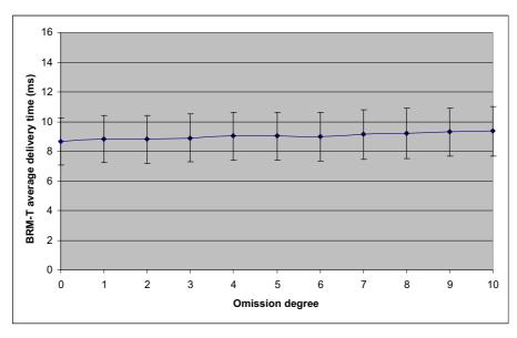
Figura 5: Six-node BRM-T average delivery time for different Od values (data size 500bytes).
