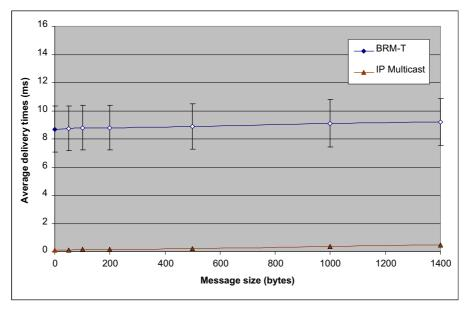
Figura 4: Six-node average delivery time for different message sizes, with Od = 2.
