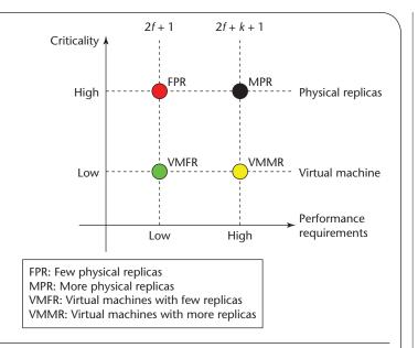
Figure 5. Deployment space for the intrusion-tolerant Crutial Information Switch. The two main dimensions are criticality (that is, the service requires tolerance to physical and software faults) and performance requirements (that is, the service requires certain performance guarantees). Implementations in this space can follow one of four main designs.
