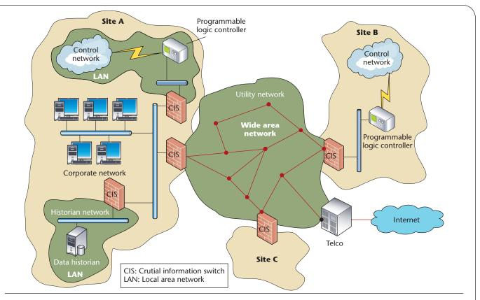
Figure 1. Crutial architecture. Crutial information switches (CISs) connect various sites' LANs to the WAN and check that all incoming and outgoing traffic meets the the host organization's security policies.
