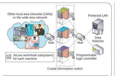
Figure 3. Intrusion-tolerant Crutial Information Switch (CIS) design. This design offers application-level policy enforcement and a rich access control model and is resilient to a fixed number of intrusions. It exploits the IPSec Authentication Header protocol using a secure wormhole subsystem on each of 2f + 1 machines to store the shared key. As with the nonintrusion-tolerant design, given enough time, an attacker could compromise the CIS machines and access the protected network.
