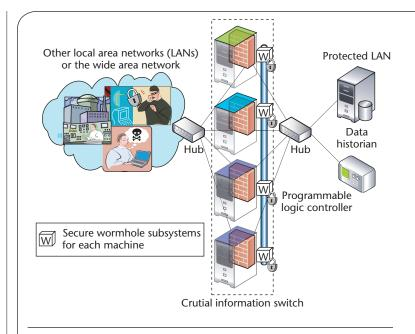
Figure 4. Intrusion-tolerant and self-healing Crutial Information Switch design. This design offers the same functionalities of the previous two designs, but adds failure-detection and rejuvenation mechanisms. A control network connects the secure wormhole subsystems in each replica machine. In this design, an attacker must compromise the machines within the recovery period and without being detected by the self-healing mechanism.
