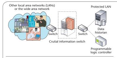
Figure 2. Nonintrusion-tolerant Crutial Information Switch (CIS) design. This design uses application-level policy enforcement and a rich access control model on a single machine to reduce the chances of an attacker deceiving the CIS with a well-crafted message and gaining access to the system. However, given enough time, an attacker could compromise the CIS machine and access the protected network.
