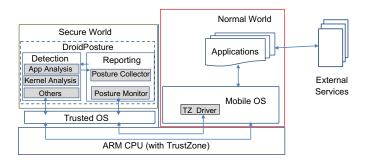
Fig. 1. Architecture of a mobile device running DROIDPOSTURE. The grey boxes are components of the DROIDPOSTURE service.
