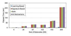
Fig. 3. DROIDPOSTURE delay when called locally with emphasis on the applications analysis modules (in seconds).
