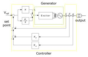
Figure 2. Automatic voltage regulator (AVR).
