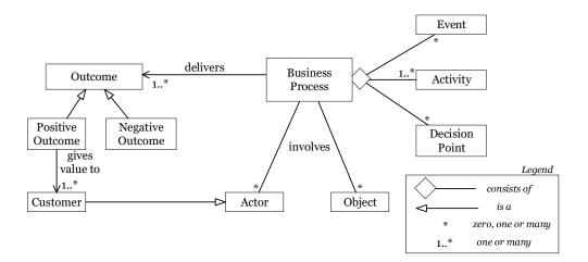
Figure 1: BPMN metamodel as proposed by Dumas et al. 2017.
