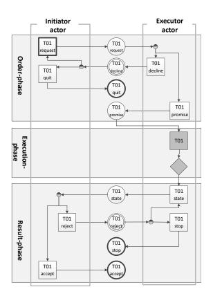
Figure 2: DEMO standard pattern of a transaction between two actors with separation between communication and production acts (Dietz and Mulder 2020).
