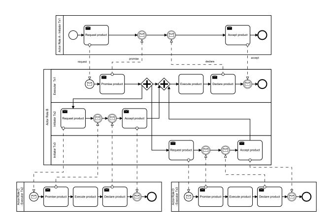
Figure 6: Dependency between transactions: request after promise pattern.
