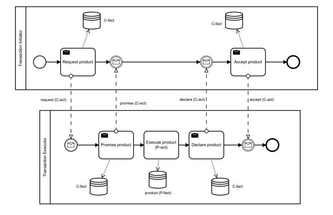
Figure 4: The DEMO standard pattern of a transaction between two actors with separation between communication and production acts represented in BPMN.
