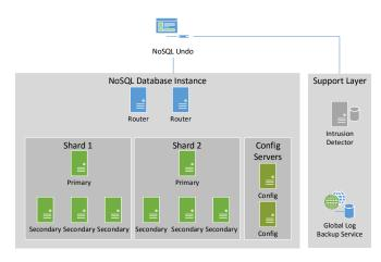
Fig. 3: A NoSQL database with NoSQL UNDO.
