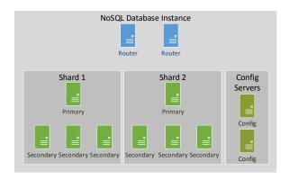
Fig. 1: Example of NoSQL instance with two shards.
