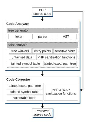
Fig. 1. Architecture of WAP with its main modules and data structures.
