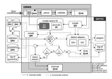
Fig. 6: Data flows for the incremental method.
