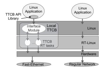
Figure 3.3: Architecture of the COTS-based local TTCB.
