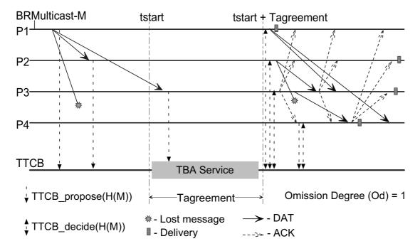
Figure 4.2: BRM-M example execution (normal case).
