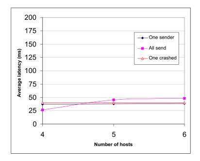
Figure 7.4: BAM-VS average latency with one sender, all sites sending and one silent site (4 sites, watermark of 10 messages, 100 bytes messages).
