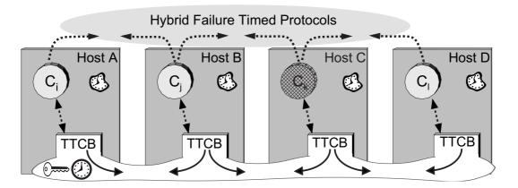
Figure 3.4: Intrusion tolerance with a TTCB.
