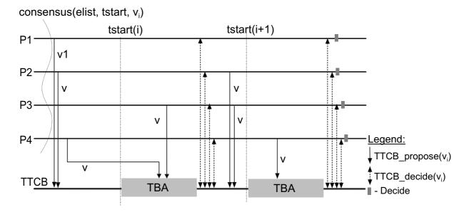
Figure 5.1: Block Consensus protocol example execution (with n=4 and f=1).
