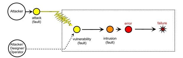
Figure 2.1: The AVI composite fault model.
