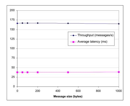
Figure 7.2: BAM-VS performance with different message sizes (4 sites, one sender, watermark of 10 messages).
