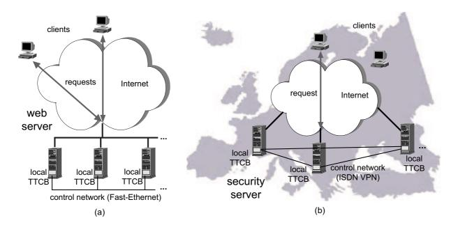
Figure 3.5: Examples of intrusion-tolerant systems with a TTCB: (a) replicated web server; (b) distributed security server.
