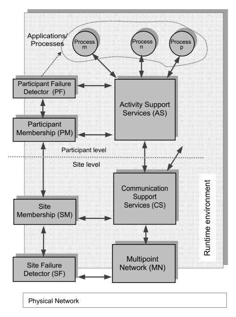
Figure 2.5: Architecture of the MAFTIA middleware in a node.
