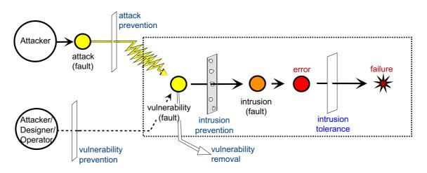
Figure 2.3: Intrusion tolerance mechanisms and the AVI model.
