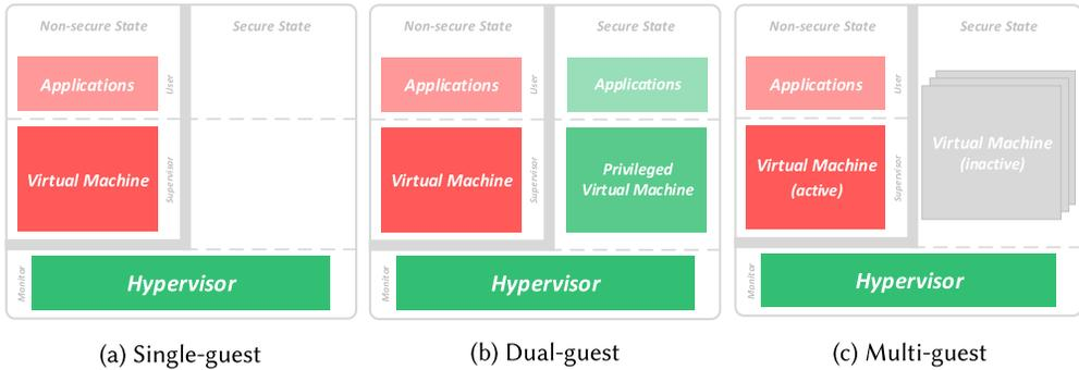
Fig. 3. TrustZone-assisted virtualization for Arm application processors (Cortex-A).
