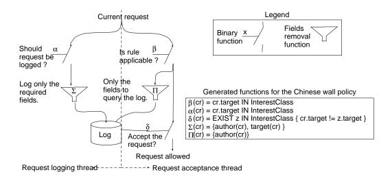
Figure 11: Schema representing the evaluation of a history-based rule.
