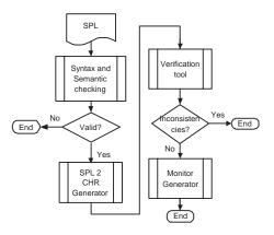
Figure 14: Overall flow of actions to generate a monitor from an SPL policy.
