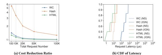
Figure 5: Simulated improvement of using IGNITE (IGN) over a no-sharing (NS) approach in: a) cost (total CPU time), and b) request latency.
