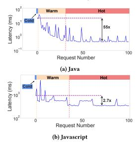
Figure 1: Latency per request for a word count (Word-Count) workload on Java and Javascript runtimes for *cold/warm/hot* stages. These runtimes improve performance by 55x (Java) and 2.7x (JavaScript) through JIT compilation and code profiling. Periodic spikes occur due to garbage collection.
