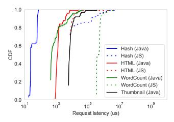
Figure 3: CDF of serverless function invocation latencies for compute-intensive tasks running on top of a Java and JavaScript runtimes.
