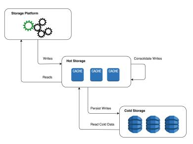
Fig. 5. Typical Storage Platform
