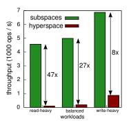
Figure 2: Performance of HyperDex with an hyperspace against a configuration with subspaces.
