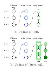
Figure 3: The chain of servers resulting from two different update operations in the same configuration of HyperDex.
